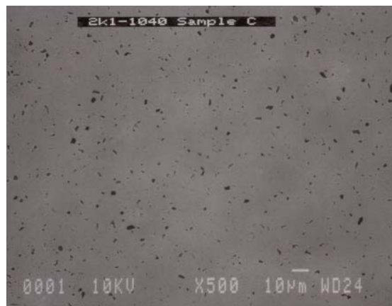
Porosity in Conventional Sintered Silicon Carbide
