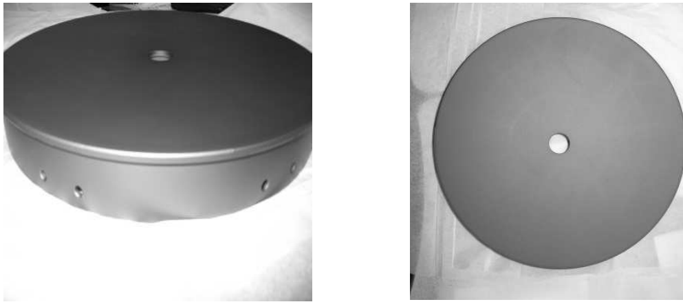
Figure 9 – Braze Before CVD segmented mirror assembly after SSiC CVD coating prior to polishing.
