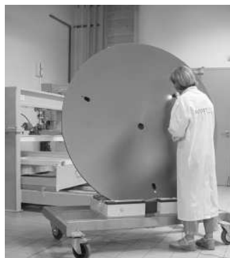
Figure 1 – Large, segmented un-coated SSiC primary mirrors; the Ø3.5m Herschel primary mirror on the left and the Ø1.5 Aladin primary mirror on the right.
