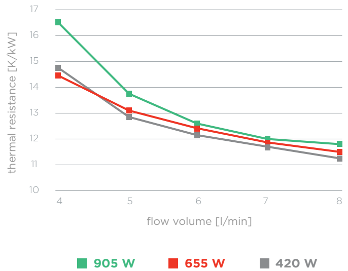
Thermal Resistance vs. Flow Volume (different wattage)
