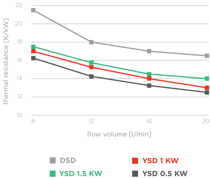
Thermal Resistance vs. Flow Volume (different diodes)
