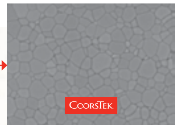
CoorsTek bonding technology. No visible bonding interface.
